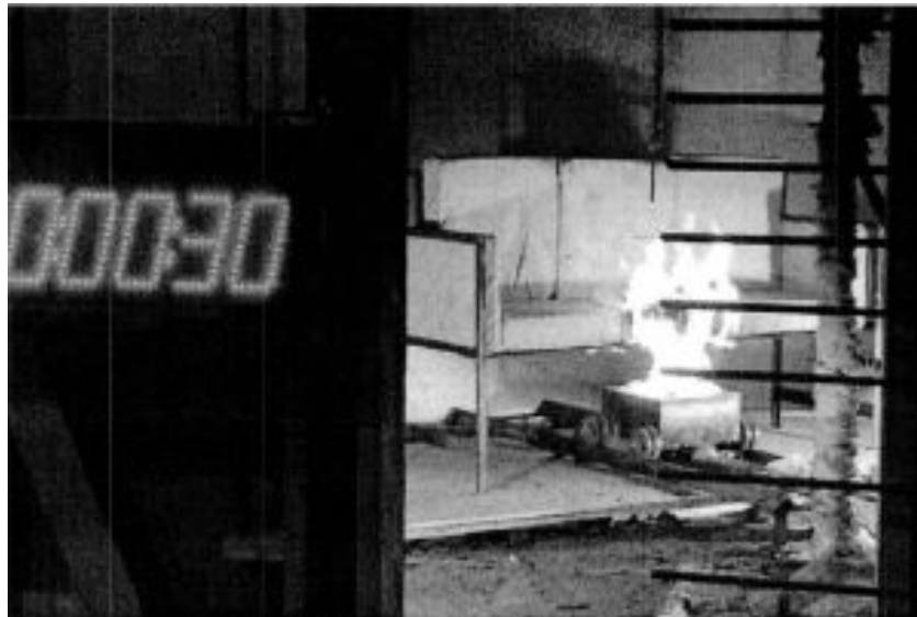
FIGURE 3.— Large-flame ignition source burner box
