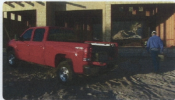
The onboard generator provides a work site with up to 50 kW of exportable power
