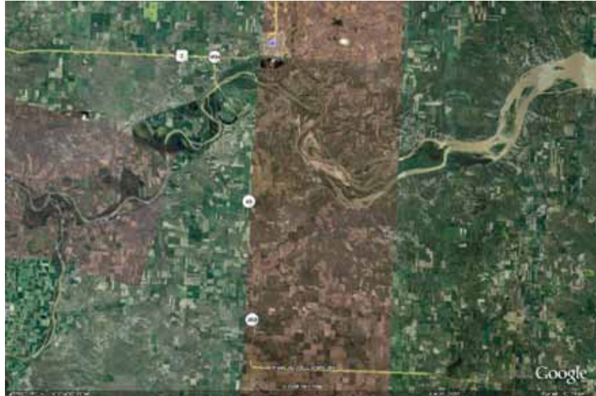
FIGURE 3-1.—Upper Lake Sakakawea area, showing sediment aggradation. (The aerial photo is from June 23, 2003 (Source: Google Earth).
