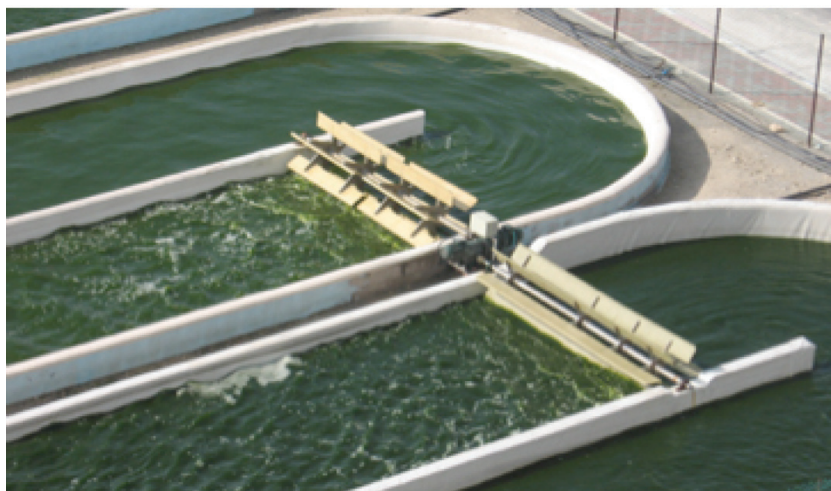
FIGURE 10.— Open Algal Cultivation System
