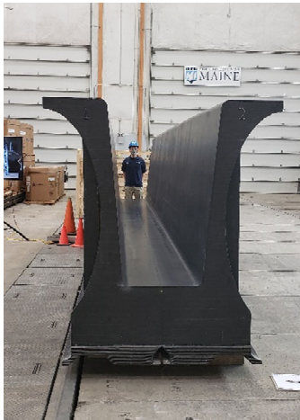
Figure 5 - 3D printed U-girder mold made on the world's largest 3D printer at UMaine.
