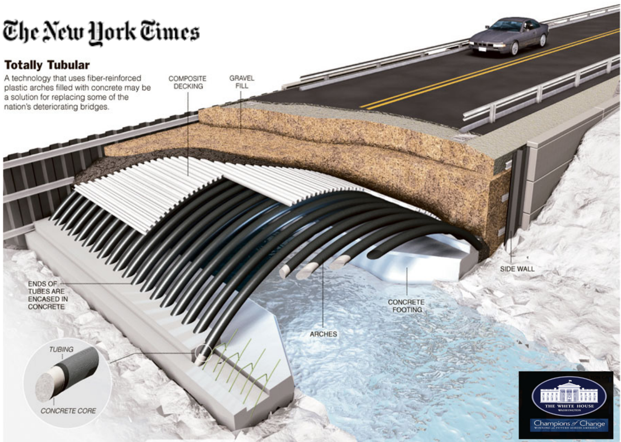
Figure 1 - Used in more than 30 bridges, the patented “bridge-in-a-backpack” technology reduces life cycle costs, reduces carbon footprint by approximately 50%, accelerates bridge construction and is AASHTO approved. Arches are lightweight and can be produced near the bridge site, which makes them suitable for disaster response. A 60 ft 2-lane bridge kit can fit on a pickup truck or in a 20 ft shipping container.
