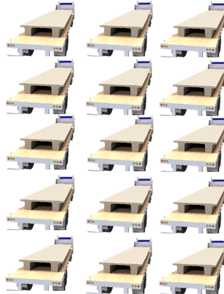
Figure 4 - Four 40ft U-girder bridges fit on one truck. The heavier concrete girders require 15 trucks.
