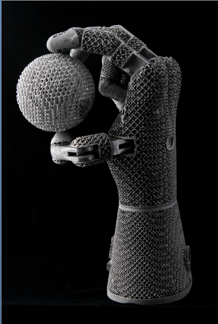
Robotic hand fabricated at Oak Ridge National Laboratory using additive manufacturing technology
